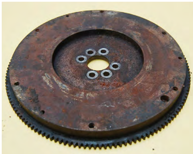
A six bolt flywheel, part no. 217250.
