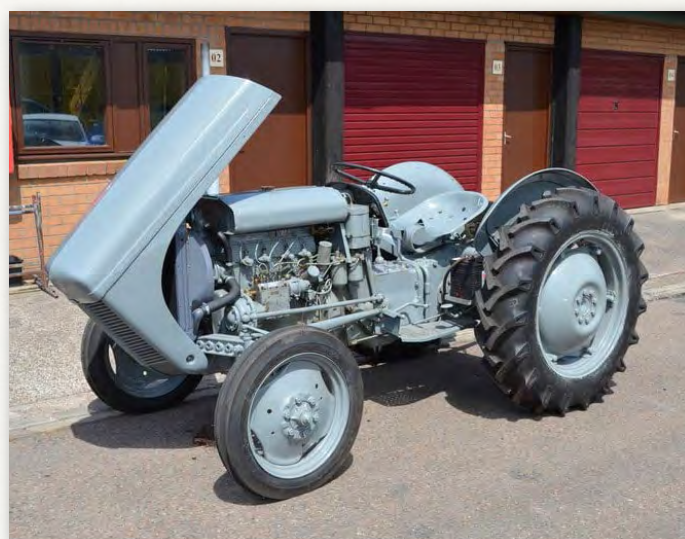
A 1956 TEF-20 with the Standard 4-cyl diesel engine. This and the last photo shows how the engine-gearbox-hydraulic casing provide the backbone, with wheels and seat hung on where suitable. Absolutely all function and little finesse!
