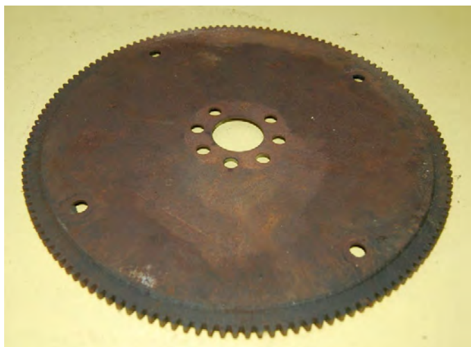
A six bolt drive plate, part no. 214766.
