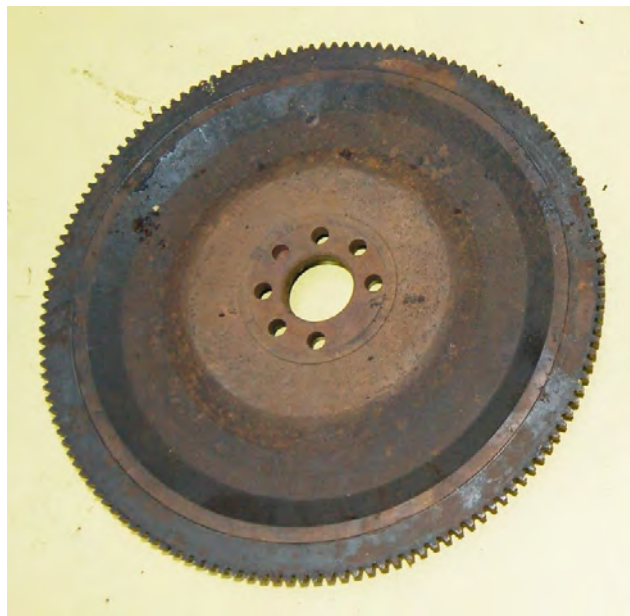
The other side of flywheel 217250 showing the join line between the flywheel itself and the detachable, shrink fit, ring gear.
