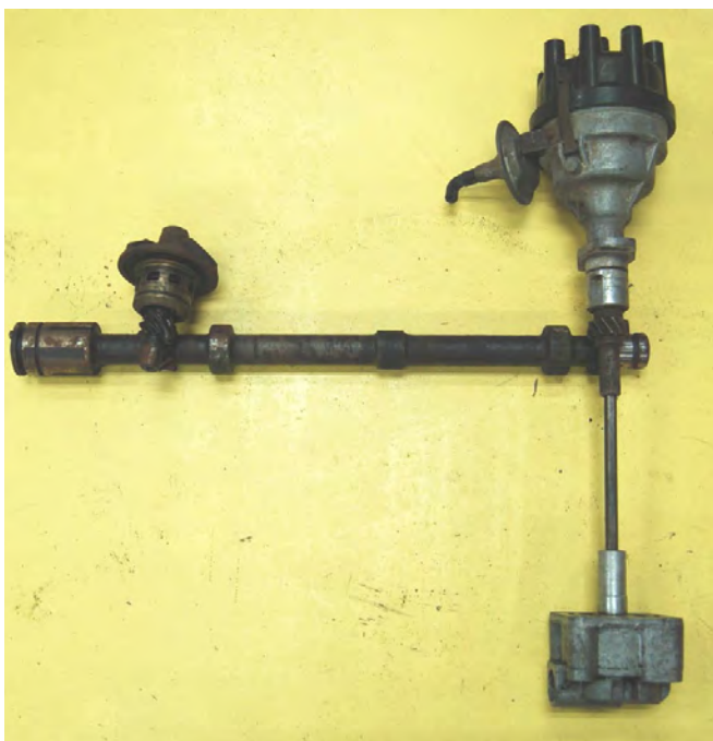
An original jackshaft (with the intermediate shoulders) showing its arrangement within the engine, driving the water pump, distributor and, through a hexagonal shaft, the oil pump.
