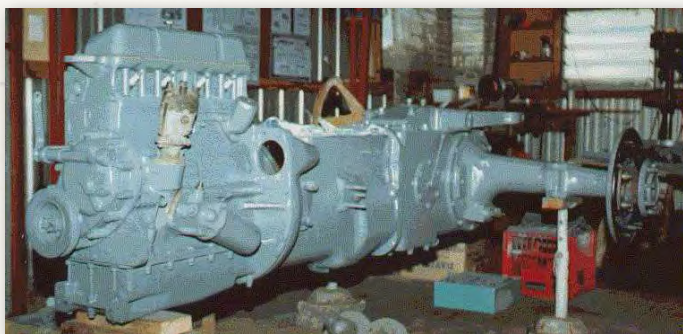
A TEA-20 engine under restoration. Obviously the petrol engine as it has spark plugs and a distributor.
