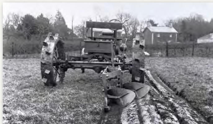
A two-furrow plough attached to a modified Model T. The rear frame has been extended and widened for the spade wheels to be fitted to and to provide a strong fixing for the attachment of the plough.
