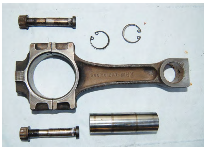
Conrod part no. 155476 with fitted bolts and the piston pin and circlips which locate the conrod in the piston.
