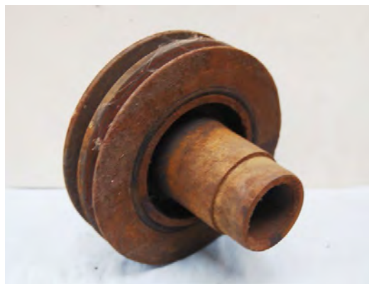
Another one of my rusty parts but this serves to show up the black rubber layer between the inner and outer steel rings which provides the damping medium.
