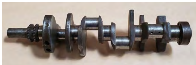
A standard Stag crankshaft – from the sprockets on the left the parts of the crank are: main bearing, large balance weight, big end bearing, small balance weight, main bearing, small balance weight, big end bearing, plain web, main bearing – then a mirror of this on the right hand side.
