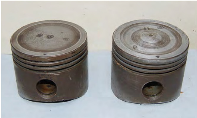
The two pistons used in UK engines, flat top 155473 on the left, domed top 160010 on the right. The arrow stamped on the front face indicates that they should be installed with this at the front and the tops are stamped with 'F' for the grade and a 3 character date in the form D76, being April 1976.
