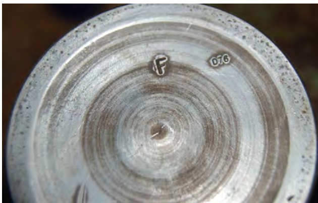
An 'F' graded piston with the date stamp top right. Note the indentation bottom left which is where a valve has hit the piston – somebody wasn't looking after their timing chains were they?
