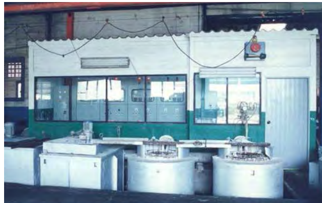
A typical Tufftriding plant using multiple immersion baths.
